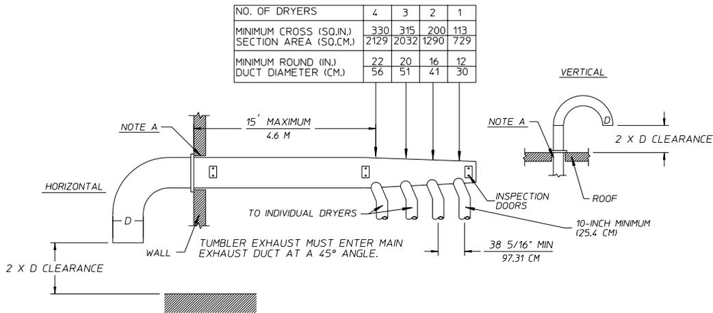
IMPORTANT: NO MORE THAN 4 DRYERS CAN BE CONNECTED TO ONE COMMON DUCT ( VENT ).
