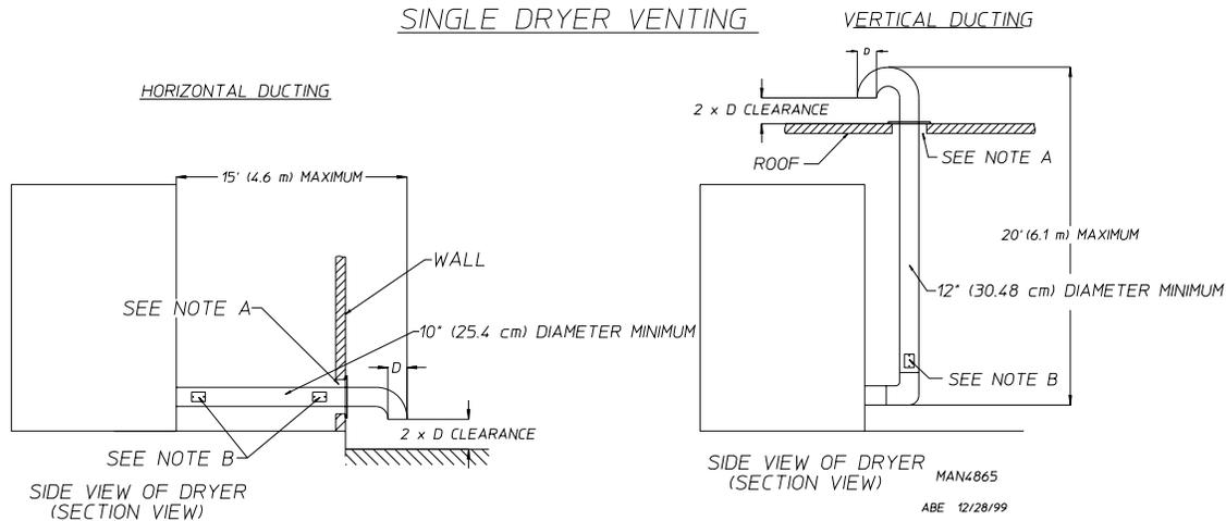
NOTE: "A"- OPENING MUST BE TWO (2) INCHES (5.08 cm) LARGER THAN DUCT (ALL THE WAY AROUND). THE DUCT MUST BE CENTERED WITHIN THIS OPENING.
