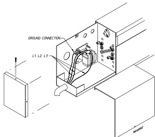
**IMPORTANT:** A strain relief **must be** used where the input wiring enters the oven assembly.
