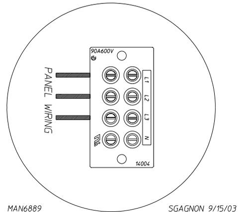
The neutral will only be used on 4-wire service. This is typical for 380-416V, 50 Hz.
